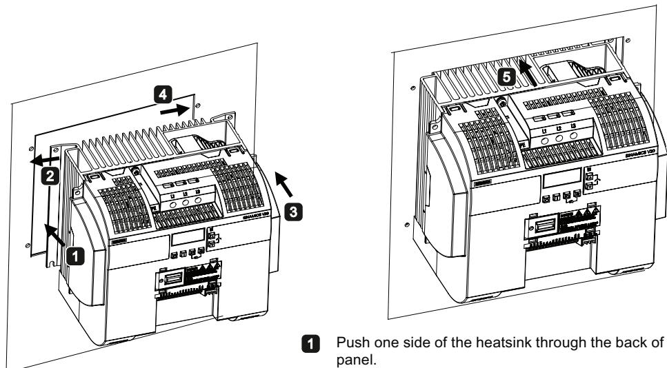
**1** Push one side of the heatsink through the back of the cabinet panel.
